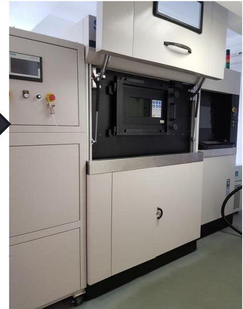
**SLA-Resin curing 3D printer
