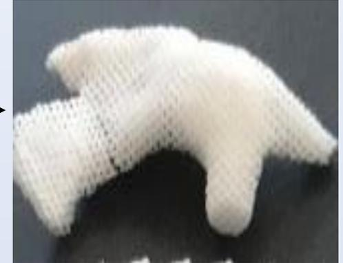
lattice structure integrated with the implant
