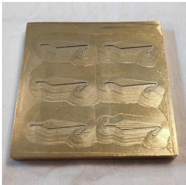
Special strategy for the mold in order to achieve the chip micrometer dimensions challenges
