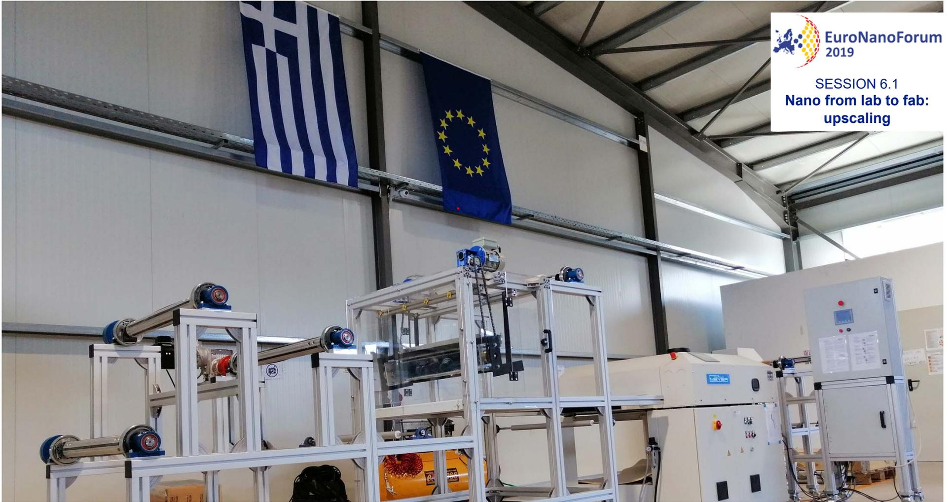
Scaling-up of Nano-enabled composite materials through a modular R2R pilot line.
