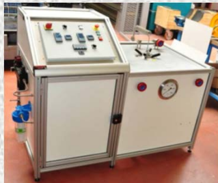
HP Systems autoclave
