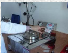
autoclave with in-situ RAMAN monitoring
