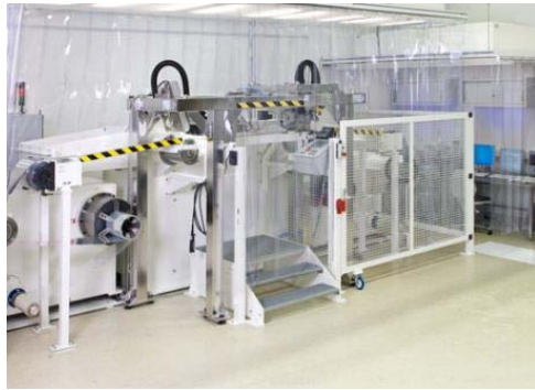
R2R surface inspection
