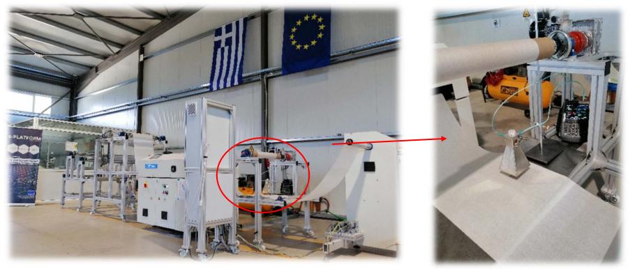
Checking how IEMN's Free Space Antenna can be integrated in ADAMANT COMPOSITES' Roll-to-Roll pilot line for nano-enabled prepregs
