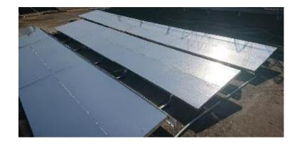
Embedded resonant polar dielectric microspheres randomly in a polymeric matrix, resulting in a metamaterial that is fully transparent to the solar spectrum while having an infrared emissivity greater than 0.93 across the atmospheric window. When backed with a silver coating, the metamaterial shows a noontime radiative cooling power of 93 watts per square metre under direct sunshine.
