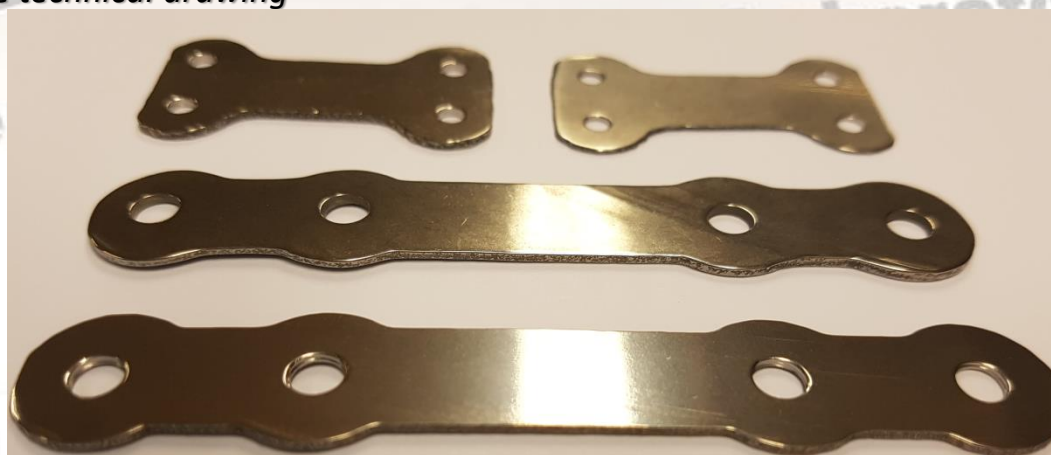
a) Technical drawing of the implant and b) Drilling of the intermediate form according to the technical drawing
