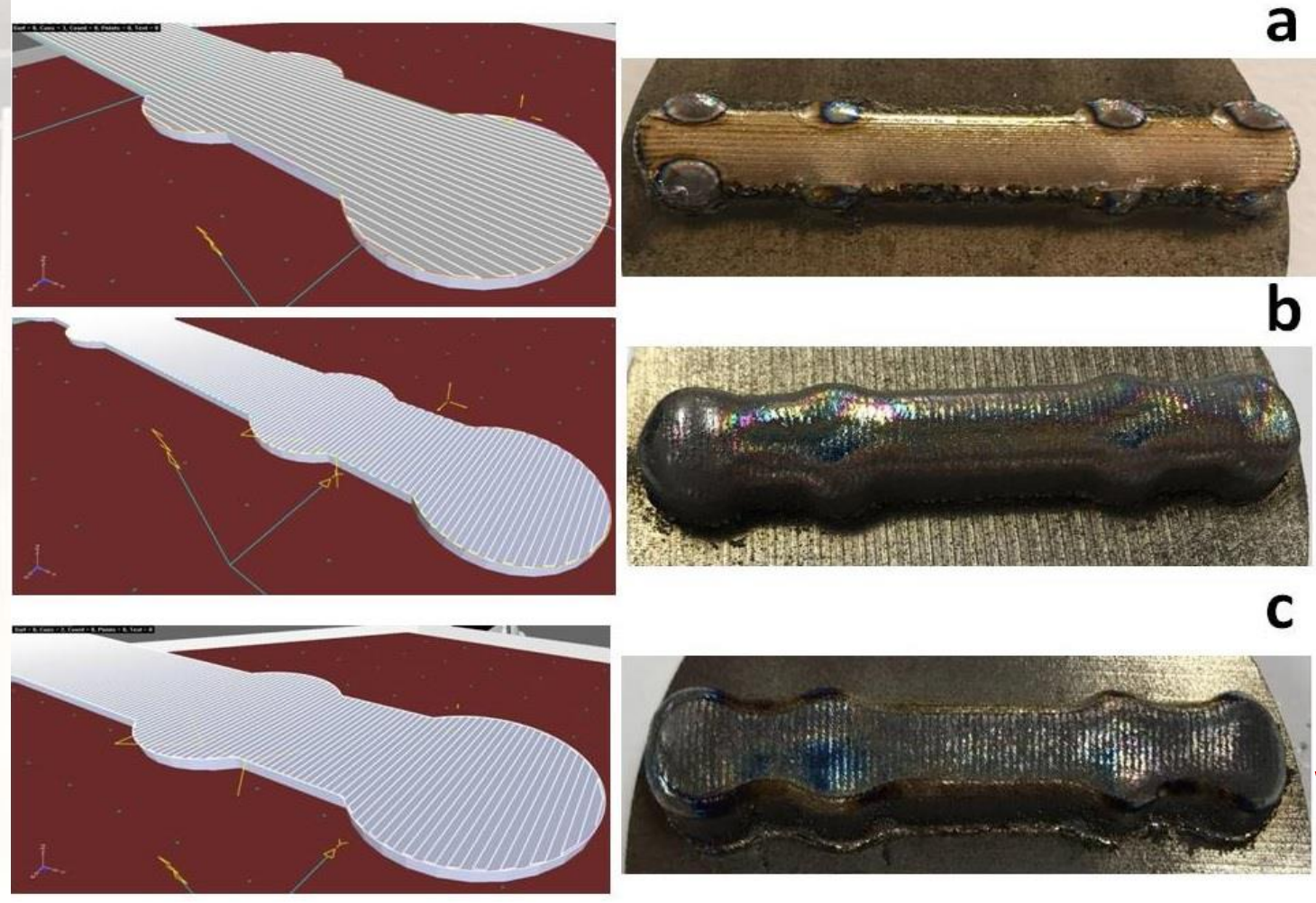
3D printing: a) cross-scanning, b) vertical scanning, and c) vertical contoured scanning
