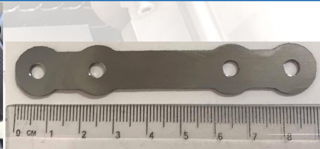
Implant according to the technical drawing produced by LMD printing followed by cutting and drilling operations
