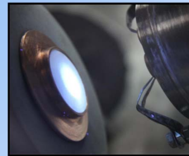
Fig. 1. Experimental principle of Coll/HAp-C.P./Zn thin films deposited by MAPLE on Ti substrate
