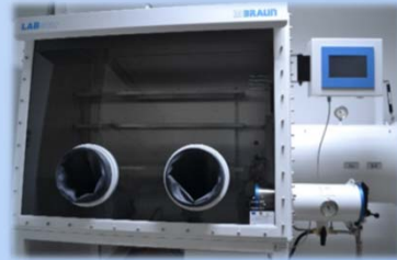
working chamber with controlled atmosphere
