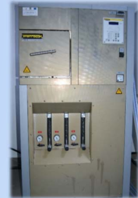
furnace for thermal treatments with connection to 3 inert gases
